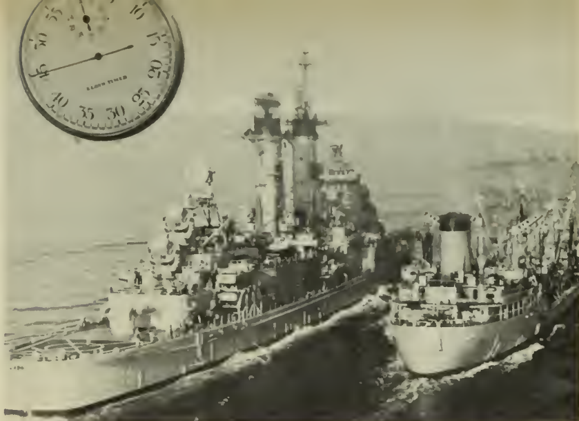
CLOCK STOPPERS — USS Albany (CG 10) claims record-breaking 45 seconds for rigging unrep refueling connections with Fleet oiler USS Chikaskia (AO 54).
